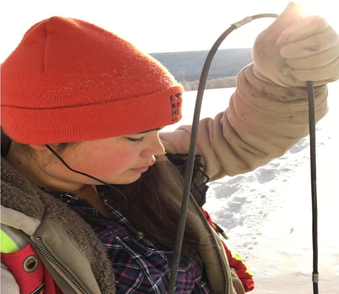
Reading Slope Inclinometers near Peace River
